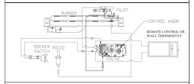
**NOTE:**Knob cannot be turned from "PILOT" to "OFF" unless knob is pushed in slightly. Do not force.
