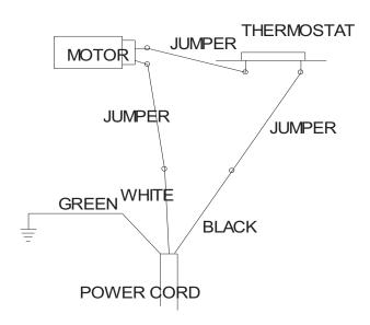
**NOTE:** If any of the original wire supplied with the appliance must be replaced, it must be replaced with a wire of at least a 105° C. temperature rating.
